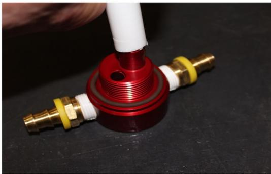
J. Place the suction tube assembly into hole. Take measurements so the bottom of the suction tube is only 1/8” (no more than 2 quarters stacked) from the bottom of the fuel tank. Before cutting the suction tube, triple check the measurements. It is more efficient to cut the tube too long and then correct to proper length than it would be to cut too short.
