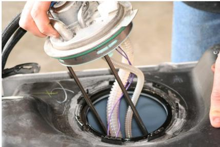
**M.** Attach 5/8" fuel line to PL-1010 and the 1/2" fuel line to the PL-1004. Remember to oil the fitting and fuel line. Loop fuel line over frame rail when reinstalling fuel tank. Do not cut at this time.
