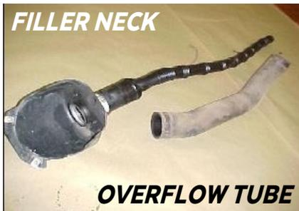
**E.** Disconnect electrical harness. Using disconnect tools, remove factory suction & return lines from fuel module. Pinch in tabs on 2011-2016. Disconnect overflow tube. You can now remove the fuel tank. To gain access to the top of the fuel tank, if necessary, carefully bend the sheet metal down that is covering the side.
