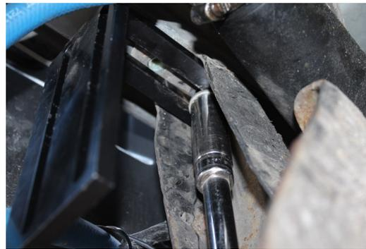
**F.** Position the PBR-2001 to the PFB-2002 pump assembly at the mounting location and check for fit. Once location is established mark location for mounting in next step.
