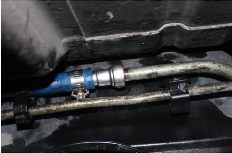
**E.** Reattach the 3 bolts holding the fuel cooler to the mounting bracket. If necessary, rebend sheet metal that allowed access to the top of the fuel tank.
