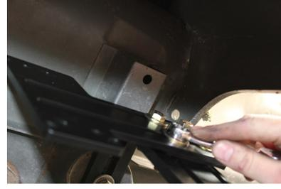
**H.** Once secure use (3) 1 1/2 bolts and (3) WA-1001D spacers to mount the pump to the bracket.
