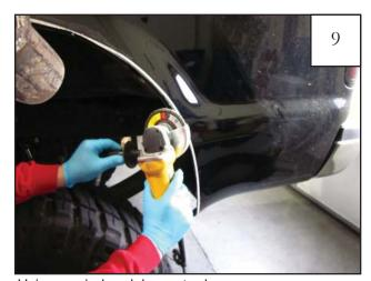
Using a grinder, debur cut edges.
