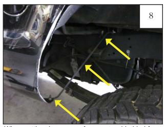
When cutting, be aware of support rod behind front side of wheel well. Angle blade inward to avoid cutting it.
