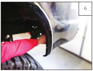
To avoid cutting the splash guard, push it into back of wheel well.
