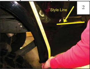
Starting from bottom under edge below mark made in previous step, measure up following curve of wheel well aproximately 15" to lower style line and mark with grease pencil.
