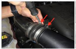
32. Reconnect the wiring harness back into the IAT sensor.
