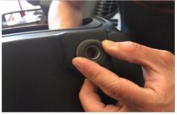
15. Install the Cuff (C) and Hose Clamp #104 (K) onto the side of the Air Box (A). Make sure that the rubber pull tab on the tube seal is on the bottom. Tighten the hose clamp.
