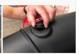
18. Install the Hump Coupler (Q) with Hose Clamp #52 (O) into the Air Intake Tube (B) that leads to the passenger side. Do not tighten the hose clamps. Install the Straight Coupler (N) and Hose Clamp #72 (P) that leads to the driver side. Do not tighten the hose clamps. To make the installation onto the turbo inlet tubes easier, try to slide the coupler in over the air intake tube as much as possible.
