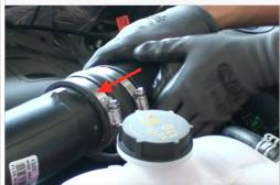
**31.** Insert the two wire harness clips disconnected in Step 11 into the holes on the side of the Air Box (A).
