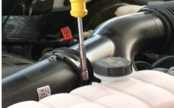
4. Loosen the hose clamp at the tube leading the turbo inlet on the driver side.
