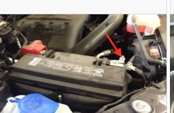
2. Loosen the hose clamp by the stock air box and pull the tube out.
