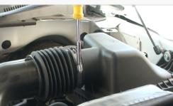
3. Loosen the hose clamp at the tube leading to the turbo inlet on the passenger side.
