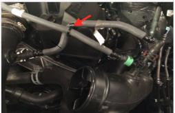
20. Install the Air Box (A). Make sure that the box prongs are aligned with the factory grommets. Push down on the air box to make sure that the prongs are completely seated.
