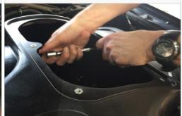
22. Install the IAT Sensor into the Air Intake Tube (B). Make sure to remove the IAT Sensor O-Ring prior to installing. Use a twisting motion to make it easier to guide the sensor into the grommet. Make sure that the sensor is seated all the way so that the sensor tab is touching the grommet and is lined up with the triangle mark located on the air intake tube.
