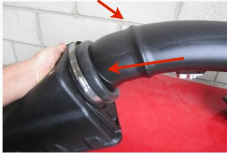
23. Once the tube is pushed flush against the stop hump of the tube the hose clamp (D) on the cuff can be tightened down. The cuff will allow some movement of the tube to accommodate engine vibration.
