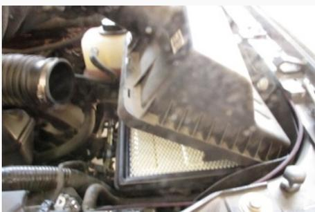
8. Remove the factory air filter.
