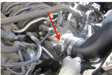
30. Connect the hardline from the engine to the hose fitting (M). Also connect the included 3/8" hose (U) to the elbow barb (T).
