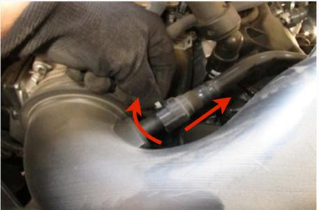
14. Disconnect the other hose toward the middle of the factory intake tube by pulling the hose off the plastic barb.
