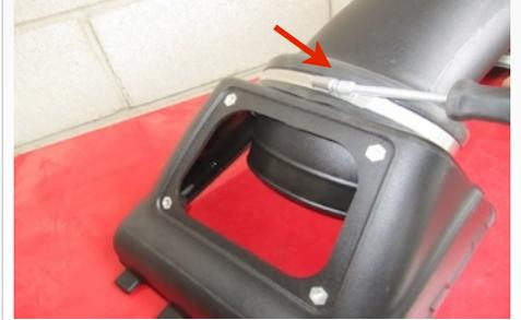
24. Install the S&B air filter (I) on to the end of the tube. Position the hose clamp (J) so that it can be accessed through the lid opening. Tighten the hose clamp.
