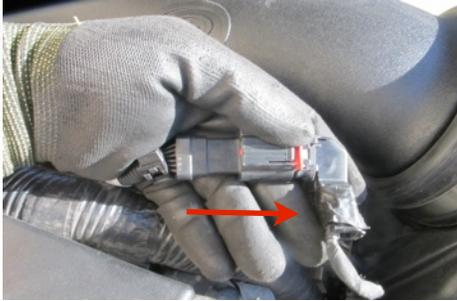
33. Connect the extension harness (V) to the factory MAF. Position the harness away from any moving or vibrating engine components.
