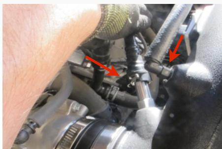
31. Connect the other end of the included 3/8" hose to the hose connector on the vehicle.
