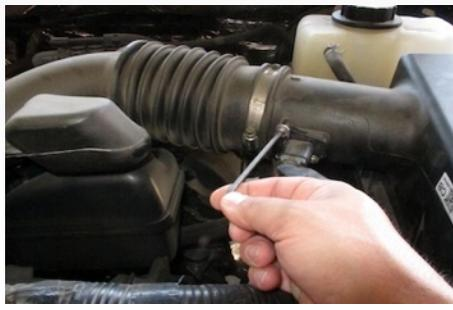
3. Once the sensor is removed disconnect the sensor from the harness by pulling the Red tab out and pressing down on the release button while pulling out. Place the sensor in a safe location for later install.
