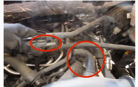
15. Loosen the hose clamp on the tube connected to the throttle body.
