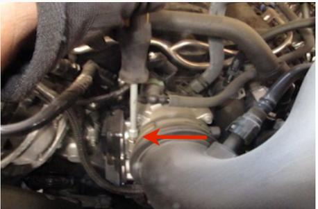
16. Once both hoses are disconnected and the hose clamp is loose on the throttle body pull the whole intake tube assembly up and out.
