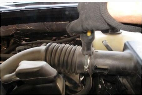
5. Once the hose clamp is loose, pull tube to the left to remove from factory air box cover.
