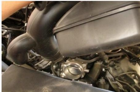
17. On the S&B intake tube (H) install both the hose fitting (M) and hose barb. (T) Install until snug and do not over tighten. **NOTE:** the orientation of the hose barb may need to be adjusted after the tube is installed.
