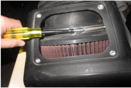
25. Install the whole intake assembly into the stock intake box. Please make sure that the tabs on the S&B air box cover fit correctly into slots on the factory box on the right hand side. Once the tabs are in the slots lower the whole intake assembly into place.
