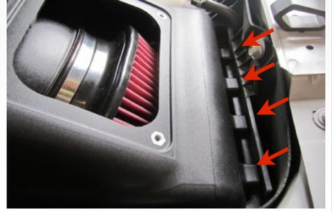
26. Lower the complete assembly and make sure the S&B Air Box Cover (B) sits inside the factory air box slots. Proper installation into the slots will reduce movement.
