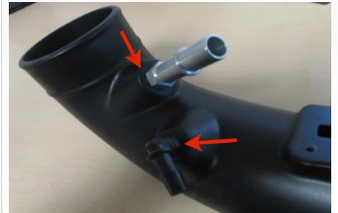
18. Install the MAF Gasket (N) then the MAF plate (O) and tighten down using the provided hardware. **NOTE:** the arrows need to point towards each other.
