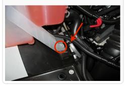
12. Remove the MAF sensor from the OE air box lid. Using the two supplied #8-32 Screws (Q) and Washer/Spacers (P), install the MAF sensor into Intake Tube (N). Do not over tighten.
