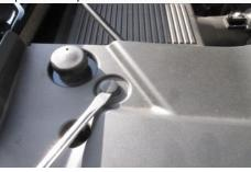
5. Remove the rubber hood seal on the passenger side by pulling forward towards the front of the hood and pulling up.
