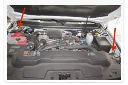
Disconnect the electrical connections for both of the Mass Air Flow (MAF) Sensor and the Humidity Sensor.
