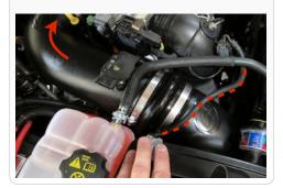
23. Slide the Hump Coupler (O) over the Intake Tube (N). When satisfied with the positioning, tighten the two #80 hose clamps (I) and #72 Hose clamp (J) at the turbo.
