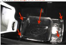
17. Once the Air Box is bolted down install the box seal (E) onto the air box.
