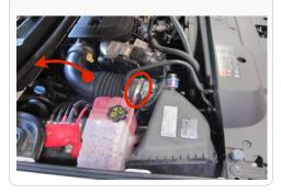
8. Remove air box lid and air filter by removing the two screws by the fender. Then carefully pull the lower portion or the air box up out of the two rubber grommets.
