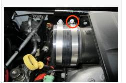
15. Move the coolant reservoir out of the way. Install the Air Box (A) flush on to the bottom of the vehicles mounting points.
