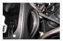
18. Slide the two #80 Hose clamps (I) over the Hump Coupler (O). Then push the Hump Coupler (O) over the Box Adapter (F). Leave clamps loose for now.
