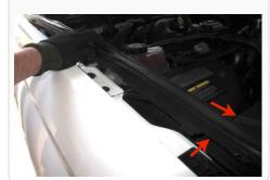
6. Remove both the upper and lower crossbars by removing the 5 mounting bolts, a 10mm & 13mm socket will be needed. The lower crossbar bolt can be accessed by pulling up on the front plastic liner
