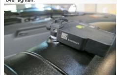
13. Remove the Humidity Sensor from the OE air box lid. Using the two supplied M4x. 7x8mm Screws (R), install the Humidity Sensor into Intake Tube (N). Do not over tighten.
