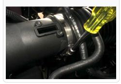
5. Once the hose clamp is loose, pull tube to the right to remove from factory air box cover.
