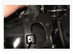
17. Remove the top bolt from the front cross bar using a 10mm socket.
