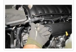
7. Once the button releases the lock pull the hose out.
