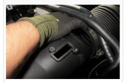
6. Remove the factory hose from the factory resonator box by first pressing in the grey button up on the bottom.
