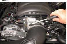
**30.** Connect the MAF harness to the MAF sensor. Make sure the red locking latch is secure.
