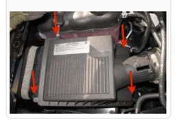
12. Remove the lid cover by lifting up and out.
