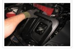
**23.** Use the provided hardware (L&K) to bolt down the S&B box to the vehicle.
