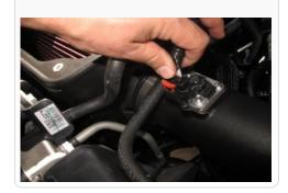
31. Use the provided Hose Clamps (V) and Crankcase Hoses (J) to install onto the S&B Intake Tube (B). Once the hoses are secure to the Intake Tube, install onto the vehicle and tighten down with the provided hose clamps (V).
