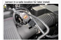
4. Use a nut driver to loosen the hose clamp on the factory air box cover.
