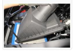
13. Remove the factory air filter.
