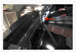
18. Remove the 4 plastic push pins on the far left side of the front liner to gain access to the front crossbar. To remove the push pins use a flat blade screw driver to pop out the top head and pull out.
