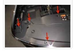
20. Lift up on the liner and remove the lower bolt using a 10mm socket from the front crossbar. Remove from the vehicle, this part will be reinstalled later.
