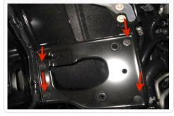
**16.** When all four bolts are removed, pull out the factory mounting plate.
