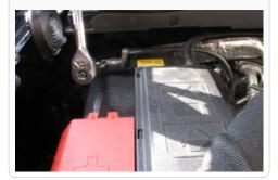
The sensor must be removed from the factory intake cover using a Torx bit.
