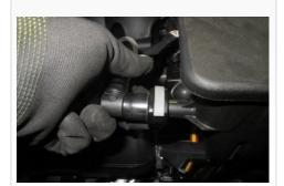
9. Loosen the hose clamp at the throttle body.
