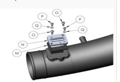
27. Use the provided hardware (P&Q) to install the Factory MAF onto the MAF Plate.
