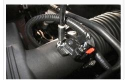
3. Once the sensor is removed, disconnect the sensor from the harness by pulling the Red tab out and pressing down on the release button while pulling out. Place the
