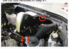
16. Remove the OE bolt that was inserted into the rubber coolant tube in Step #6 and push the tube end over the end of the 90deg. Hose Barb (E).
