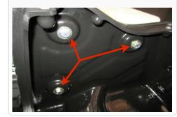
15. Install the Air Box/ Coolant Tank assembly into the truck. Push the prongs on the bottom of the air box into the OE grommets set in the frame. Secure the using the OE bolt removed in Step #7.
