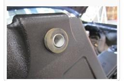
11. For those concerned about minimal engine heat; insert the three Clip Nuts (T) over the holes on the bottom opening of the Air Box (A), insert the Box Plug (U) into the end of the Air Box (A). Attach using the supplied 1/4-20 Hex Screws (V) and Flat Washers (Y) from the inside of the Air box using 5/16" socket or ratcheting wrench. For those seeking additional air flow, set the Air Box End Cap aside. (See page 4 for more info)
