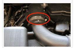
3. Disconnect the MAF sensor by sliding the red locking pin back, press in the bottom of the harness and pull out the male connection.
