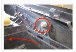
8. Pull the assembly out of the factory grommets and remove from truck. Note: You will have to remove the bolt from the rubber tube to fit through the air box assembly.
