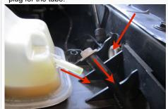
7. Remove the other air box mounting bolt using 13mm socket. Carefully tip the air box assembly away from the fender so that coolant isn't spilt.
