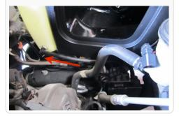
17. Remove the coolant from the OE reservoir and pour it into the Coolant Recovery Tank (B). Note: It may be necessary to add coolant to meet fill range of the new tank. Be sure to use Ford approved coolant. (See Page 4 for more info)
