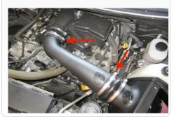
24. Install the supplied MAF sensor extension harness (Z) between the MAF sensor and the OE MAF connector. Use the supplied wire tie to position the harness away from any potential hazards.
