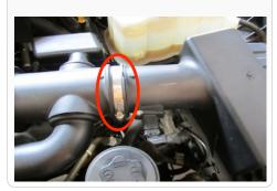
5. Undo the three clips holding the air box cover to the air box. Remove the air box lid and air filter from the truck.
