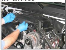
3. Disconnect the electrical connection to the MAF sensor at the OE air box.
