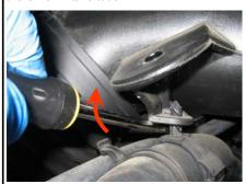
6. Loosen the hose clamp at the throttle body and at the MAF sensor and remove the OE intake tube from the engine
