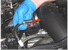
**21.** Reconnect the MAF sensor electrical connection.
