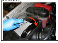
**13.** Connect the MAF sensor assembly to the S&B Filter Adapter ( I ) and secure using a # 60 Hose Clamp (J).
