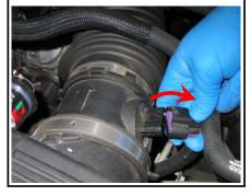
4. Pull the crankcase vent line from the OE intake tube and then from the engine along with the rubber hose connector and remove it from the vehicle
