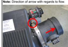
**9.** Remove the OE air box tray from the vehicle. Four of these bolts if long enough, may be used to secure the S&B air box to the vehicle. If not use the supplied M6 allen head screws (K) and SS washers (R).
