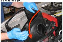
**15.** Slide the S&B Throttle Body Adapter (O) over the S&B Tube (M) along with the #72 Hose Clamp (N), do not tighten at this step.
