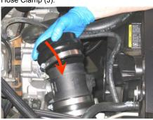
**18.** Place the S&B Air Filter (D) into the S&B Air Box (G), rotate the filter about a 1/4 turn for clearance and slide onto the flange and secure the # 80 Hose Clamp (E).
