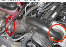
7. Pull the OE air box towards the engine and up to release it from the vehicle.
