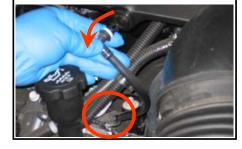
Carefully pry the hose router clamp from the OE air intake tube.
