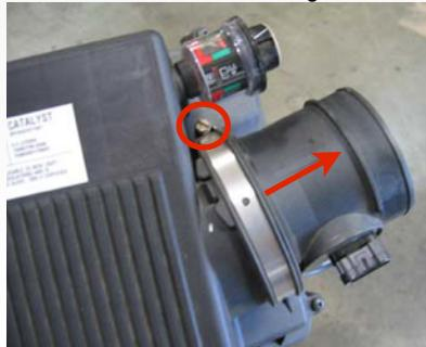
**9.** Remove the OE air box tray from the vehicle. Four of these bolts if long enough, may be used to secure the S&B air box to the vehicle. If not use the supplied M6 allen head screws (K) and SS washers (R).
