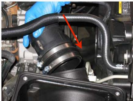
14. Slide the S&B Hump Adapter (L) over the MAF sensor's flange and secure using a # 60 Hose Clamp (J).
