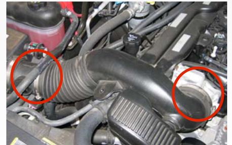
**7.** Pull the OE air box towards the engine and up to release it from the vehicle.
