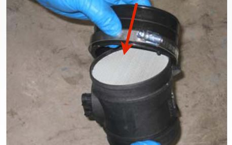
13. Connect the MAF sensor assembly to the S&B Filter Adapter (I) and secure using a #60 Hose Clamp (J).
