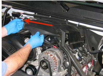
**3.** Disconnect the electrical connection to the MAF sensor at the OE air box.
