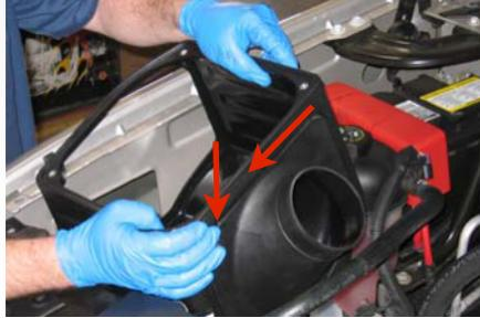
12. Slide the S&B Straight Adapter (F) over the MAF sensor's honey comb end, secure using a # 60 Hose Clamp (J).
