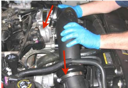
17. Install the Crankcase Vent Hose (Q) onto the S&B Intake Tube (M) vent port and then onto the engine port where the OE line was removed in step #4 . Secure with two # 4 Hose Clamps (P).
