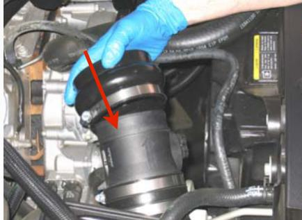
15. Slide the S&B Throttle Body Adapter (O) over the S&B Tube (M) along with the # 72 Hose Clamp (N), do not tighten at this step.
