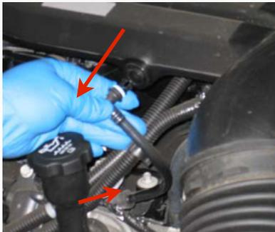
**5.** Carefully pry the hose router clamp from the OE air intake tube.
