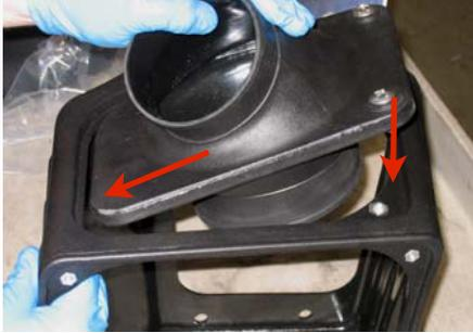
11. Place the S&B Air Box assembly into the vehicle, align the 4 holes with the OE mounting locations and secure using either the OE bolts or the supplied M6 allen head screws (K) and SS washers (R).
