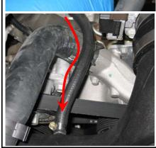
**12.** Attach the MAF sensor to the S&B filter adapter (I), secure with #60 hose clamp (K). **Note:** Direction of the air flow.
