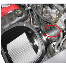
**15.** Install the S&B tube (O). Place the hump adapter end over the MAF and secure the #60 hose clamp. Then place the other end with the step adapter (P) over the throttle body and secure the #64 hose clamp (S).
