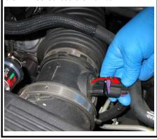
Loosen the hose clamp at the throttle body and at the MAF sensor, remove the OE intake tube from the engine
