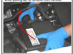
2. Pull up and out to remove the engine cover from the vehicle.
