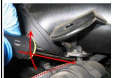
8. Loosen the hose clamp on the OE air box and remove the MAF sensor.
