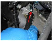
**14.** Install the S&B step adapter (P) to S&B tube (O) as shown, secure the #72 hose
