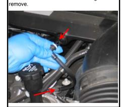
Slide the OE air box towards the engine while pulling up, to remove from vehicle.
