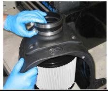
**13.** Place the S&B hump adapter (M) over the S&B tube (O), slide on until rib on tube is captured by the groove in the adapter. Then secure with #60 hose clamp (K).
