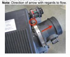
9. Place the S&B filter (D) inside the S&B air box (H), then attach the filter adapter (I) to the box using the 5/16 screws (J).
