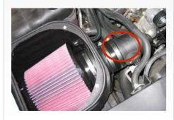
13. Place the S&B hump adapter (M) over the S&B tube (O), slide on until rib on tube is captured by the groove in the adapter. Then secure with #60 hose clamp (K).
