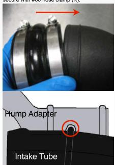
14. Install the S&B step adapter (P) to S&B tube (O) as shown, secure the #72 hose clamp (R).
