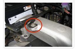
4. Remove the lock nut and pull the prong out that secures the wiring harness to the elbow and push the harness back away from the elbow.
