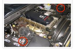
2. Loosen the upper hose clamp at the OE elbow and disconnect the hump hose from the elbow. **Note:** Care should be taken not to let any debris fall into the boost tube.
