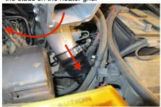
16. Install the two M8 Socket head screws (E) and M8 washers (D) through the two holes . Hand tighten for now.
