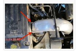
17. Place a M8 washer (D) over each stud and thread on the M8 lock nuts (C). Torque both the lock nuts and the screws to 145 ln. lbs. If you use a crow foot to torque the nuts, see the crow foot calculation on page 3. If there was a ground wire connected to the manifold, place it back in the same location.
