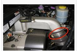
3. Remove the bolt that secures the dip stick tube to the elbow.
