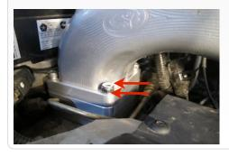
18. Slide the OE t-bolt clamp up onto the Silicone adapter (O) and torque the clamp to 90 ln. lbs.
