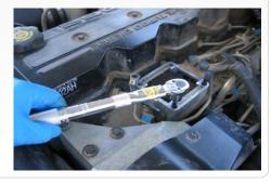
11. Apply a thread sealant such as Teflon tape to each 1/8" NPT plug (G) and insert the plugs into the ports you will not use on the S&B elbow. Use a 3/16 hex socket and tighten, do not exceed 40 ln. lbs.
