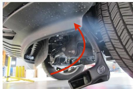
**9.** From inside the air box grab the top of the Scoop assembly and align with the three holes in the air box. **Note:** It is necessary to move some wiring harnesses out of the way to gain clearance for the scoop assembly.
