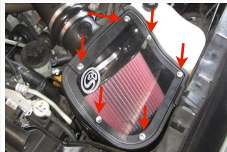
18. Reconnect the negative battery terminal. Inspect the installation, be sure the kit is properly positioned and all fasteners are secure.
