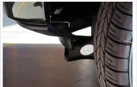
19. Check to make sure the Scoop assembly does not interfere with the wheel or wheel well liner. Turn the wheel in both directions while trying to simulate full suspension travel.
