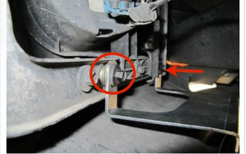
13. Attach the Mounting Bracket (F) to the Scoop Base (D) using the two supplied 5/16" Bolts (H), four 5/16" Washers (G), and two 5/16" Nuts (I).
