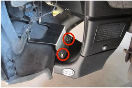
14. When you are satisfied with the position of the scoop, tighten all the 5/16" hardware using 1/2" socket on top and a 1/2" wrench on the inside.
