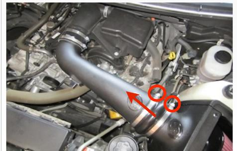
**4.** If installed, remove the air box plug from the air box. If not, install the three clip nuts that were supplied with the intake kit onto the bottom opening lip of the air box.
