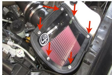
**3.** Loosen both hose clamps on the hump adapter and slide the hump adapter over the intake tube. Then remove the Adapter tube and Air Filter from the air box.
