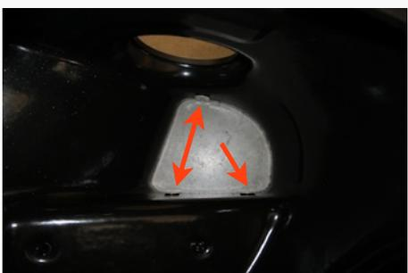
**5.** Install the three Clip Nuts (E) over the holes on the Scoop Base (D) as shown.
