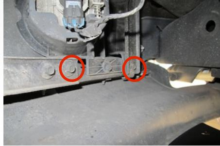
12. Attach the Mounting Bracket (F) to the bumper bracket using three Flat washers (G) and the OE bolt for the left side tab and just the OE bolt on the right side tab. Tighten both bolts.
