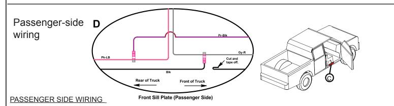
1. Remove passenger side front sill plate, open wire bundle and locate rear door-ajar wire (pink with light bllue stripe). This wire will be located rear of junction where wires route under from passenger seat.
