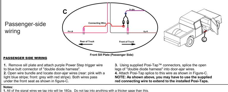
2. Occasionally the wire colors do not match the wire schematics. Under these circumstances you will need to locate the door-ajar signal wires. Each door will have one wire leading out to its latch and one ground wire coming away. The ground wire will usually be solid black. The signal wire we need is the other wire. 3. Make sure you secure all wires after install. Loose wires can be damaged and may cause a failure in the Powerstep's function.
