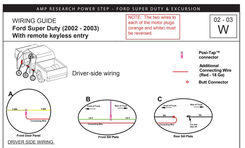
1. Remove front door panel and locate bundle of wires below and to the left of speaker (Area-A). Open bundle and locate 18 Ga door-ajar wire (yellow with black stripe).
