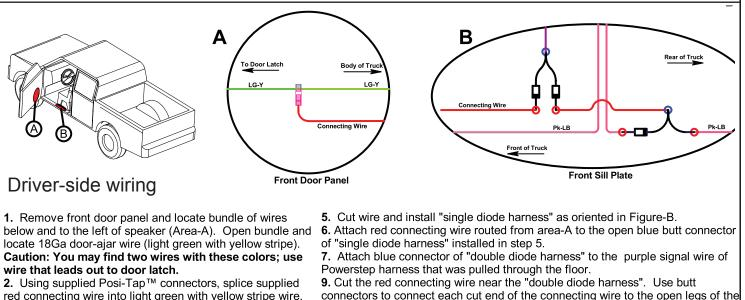
2. Osing supplied Post-Pap Connectors, splice supplied To S. Out the rou connecting vire into light green with yellow stripe wire.
