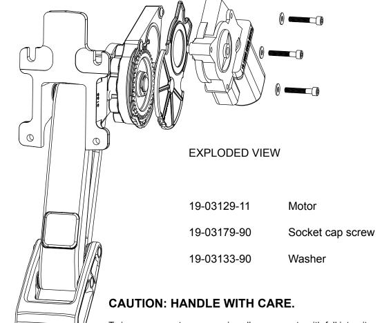
To insure our customers receive all components with full integrity, we pack the motors seperate from their linkage assemblies. This requires that the installer position and fasten the motor before continuing with the install. Please follow the instructions below and handle the assembly carefully.
