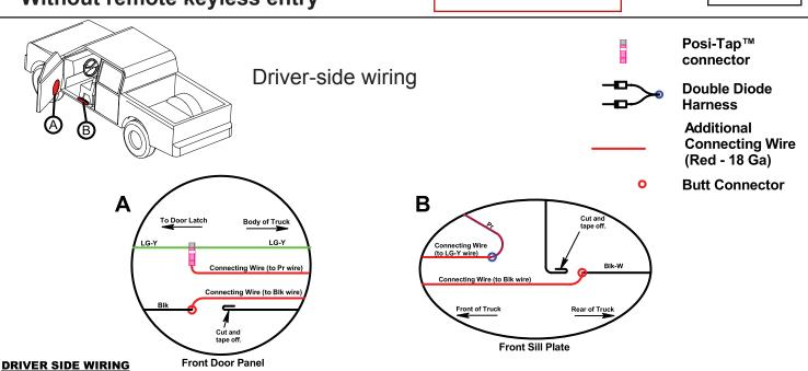
1. Remove door panel, access a bundle of wires below and to the left of speaker (Area-A). Open bundle and locate 18Ga. door-ajar wire ( light green with yellow stripe).
