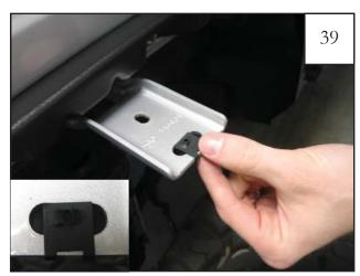
Before installing the outer flare, install speed clip on metal frame angle support bracket at top center of wheel well. Make sure that it is centered over the factory slot with threaded portion facing up.
