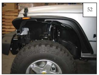
Completed front driver's side flare installation.
