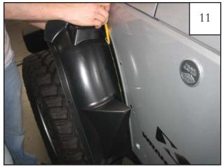
Using sheet metal as guide, mark the rear portion of the splash shield with a grease pencil in preparation for trimming. The splash shield should be flush with the sheet metal after being trimmed. *NOTE: If trimmed too little, flare won't fit; if trimmed to much, shield won't stay behind flare.*
