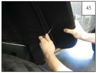
Hold flare in place on fender and start a pan head screw into each hole location and through speed clip on inner structure and metal frame angle support bracket (7 places). Do not tighten.
