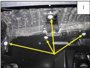
Using a socket wrench with a 10mm socket, remove four factory bolts from inside of splash shield. Save bolts for reinstallation.
