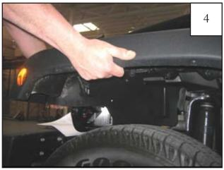
Starting at front of flare, pull *firmly* to release flare and splash shield from fender, working your way to the back. You will hear popping noises as clips release. It is okay. If clips break, they will be discarded.
