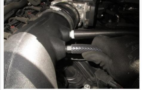
36. Connect the other end of the provided 3/8" hose to the vehicle hose connector.
