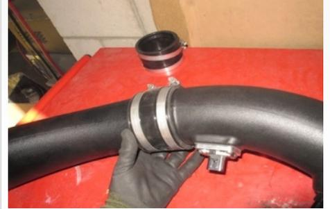
25. Install the cuff (G) onto the S&B air box cover (B) making sure that the tab on the cuff aligns with the notch on the S&B Air Box Cover.
