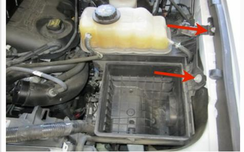
13. Near the stock resonator box loosen the hose clamp.
