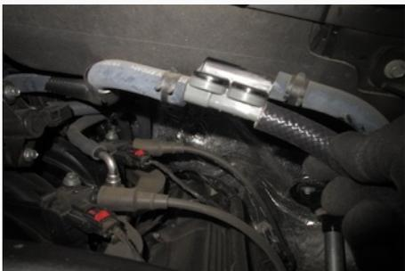
37. Connect the extension harness (Y) to the vehicle connector. Zip Tie away from any moving parts.
