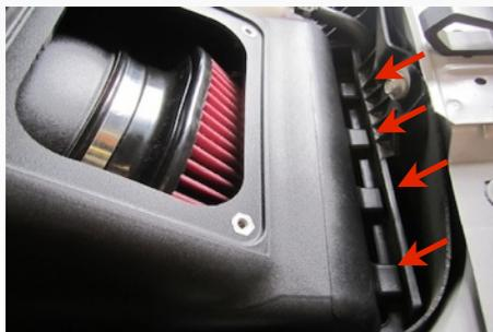
29. Lower the complete assembly and make sure the S&B Air Box Cover (B) sits inside the factory air box slots. Proper installation into the slots will reduce movement.
