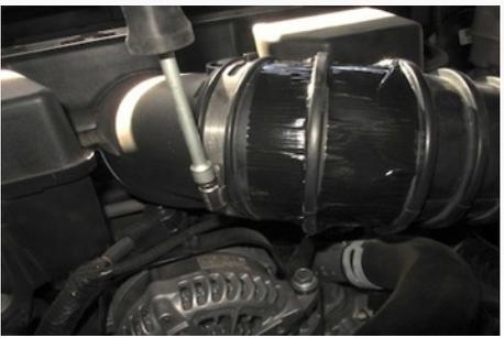
14. Remove the tube from the vehicle by pulling out.
