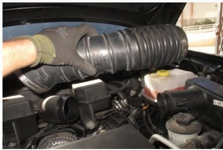
15. On the right side of the stock resonator box remove the rubber tubing from the box by pulling out and away.
