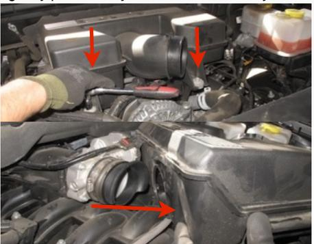
20. Remove the stock rubber boot from the throttle body.
