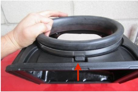
26. Insert the intake tube (W) into the cuff (G). Please make sure that the tube is pushed all the way to the stop hump of the tube. Tighten hose clamp (H).
