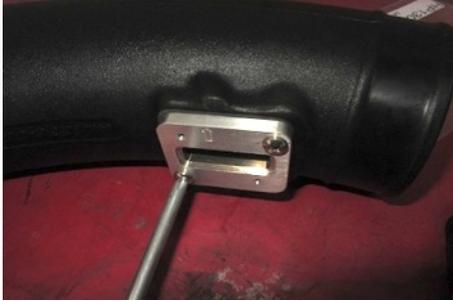
23. Install the factory MAF onto the MAF plate (N) using the provided hardware (P & Q).
