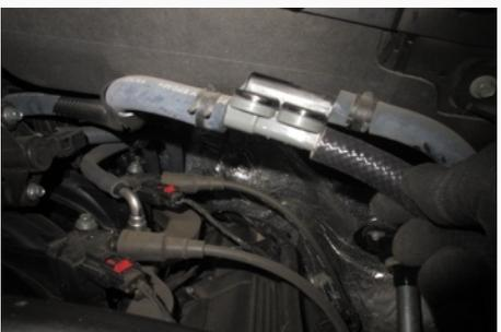
17. Remove the second hose from the box also, to disconnect the connector slide the white tab counter clock wise to release the lock.
