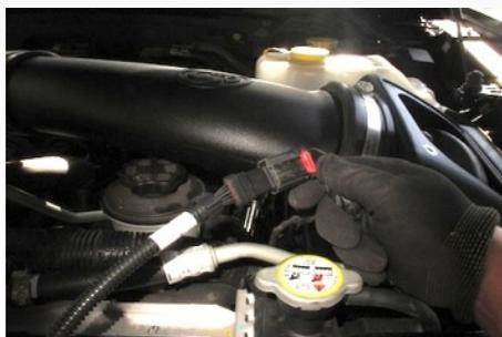
38. Connect the extension harness to the vehicles MAF. Remember to lock the red latch.
