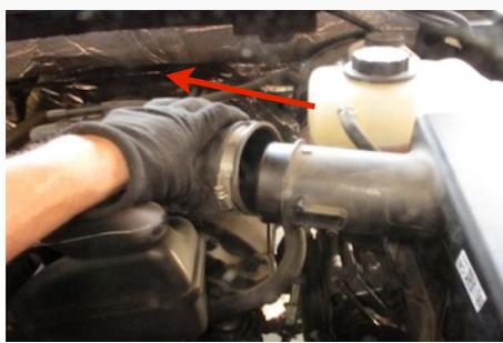
6. Remove the factory air box cover by disconnecting the three metal latches that are on the side of the factory air box.
