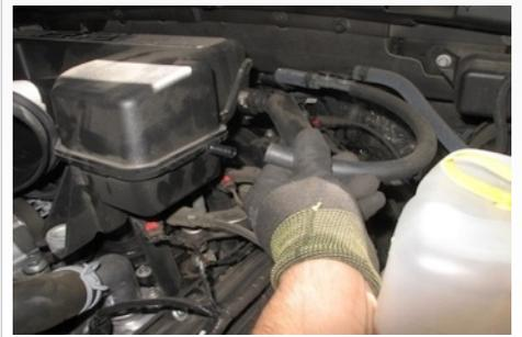
16. Remove the tube from the hose line connector.
