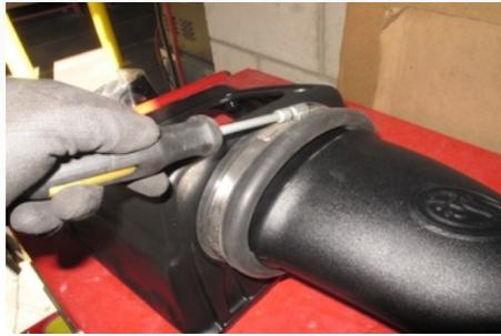
27. Install the S&B air filter (D) on to the end of the tube. Position the hose clamp (E) so that it can be accessed through the lid opening. Tighten the hose clamp.
