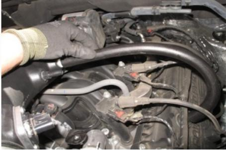
34. Use the provided hose clamp (Z) to tighten down the hose on the engine side.
