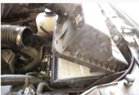
8. Remove the factory air filter.
