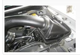
29. Lower the complete assembly and make sure the S&B Alr Box Cover (B) sits inside the factory air box slots. Proper installation into the slots will reduce movement.
