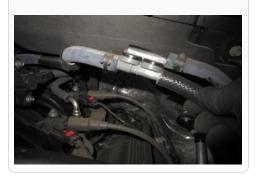
37. Connect the extension harness (Y) to the vehicle connector. Zip Tie away from any moving parts.
