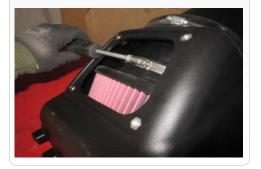
28. Install the whole intake assembly into the stock intake box. Please make sure that the tabs on the S&B air box cover fit correctly into slots on the factory box on the right hand side. Once the tabs are in the slots lower the whole intake assembly into place.
