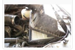
8. Remove the factory air filter.
