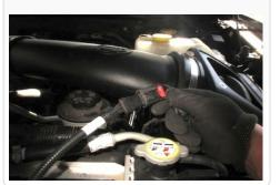
38. Connect the extension harness to the vehicles MAF. Remember to lock the red
