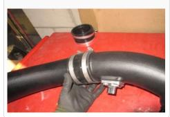
25. Install the cuff (G) onto the S&B air box cover (B) making sure that the tab on the cuff aligns with the notch on the S&B Air Box Cover.
