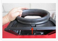
26. Insert the intake tube (W) into the cuff (G). Please make sure that the tube is pushed all the way to the stop hump of the tube. Tighten hose clamp (H).
