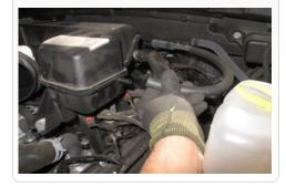
18. Remove the tube from the engine which also has a locking tab that needs to be unlocked.
