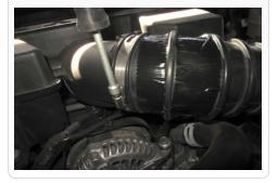
**16.** Remove the tube from the hose line connector.
