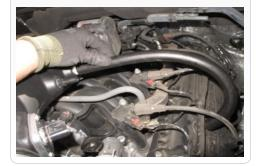
**34**. Use the provided hose clamp (Z) to tighten down the hose on the engine side.
