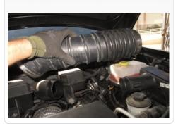
17. Remove the second hose from the box also, to disconnect the connector slide the white tab counter clock wise to release the lock.
