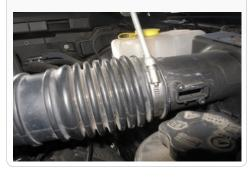
5. Once the hose clamp is loose, pull tube to the left to remove from factory air box cover.
