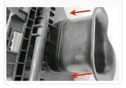
**14.** Remove the tube from the vehicle by pulling out.
