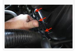
**31.** Fasten the air box lid (F) using the provided hardware (K & L).
