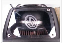
**32.** Slide the coupler (C) over the throttle body and tighten the hose clamp (I) on tube (X). Some slight adjustments may need to be made to acquire proper alignment of both
