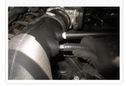
36. Connect the other end of the provided 3/8" hose to the vehicle hose connector.
