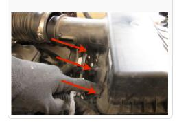
7. Once all three latches are disconnected, lift the cover up and remove from truck.
