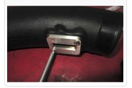
23. Install the factory MAF onto the MAF plate (N) using the provided hardware (P & O).
