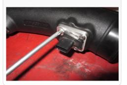
24. Connect both tubes (X & W) using the coupler (C) and hose clamps. Leave the hose clamps loose to allow for adjustments.
