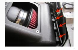
$\label{eq:28.Fasten the air box lid (E) using the provided hardware (F&G).$
