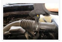
7. Once all three latches are disconnected, lift the cover up and remove from truck.
