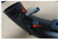
**20.** On the opposite side of the intake tube, install the coupler (K) and hose clamps (L). Only tighten down the hose clamp on the tube side leaving the throttle body side loose for install.
