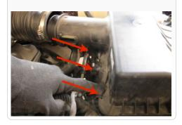
9. Move the factory air box by removing both bolts and lifting up on the box. This is required to gain access to the side inlet.
