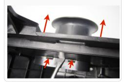
**11.** Install the S&B fender Inlet (W) by pushing in firmly until it snaps into place.
