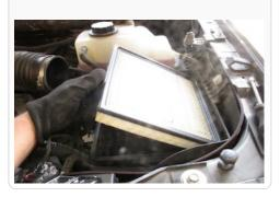
8. Remove the factory air filter.
