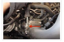
**18.** Install the MAF Gasket (N) then the MAF plate (O) and tighten down using the provided hardware. NOTE: the arrows need to point towards each other.
