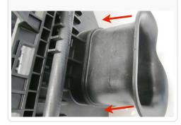
12. After the S&B inlet is installed, lower the factory air box back down and reinstall the factory bolts. Make sure the S&B inlet (W) is pushed through the side skirt.
