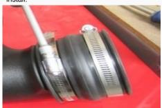
15. Loosen the hose clamp on the tube connected to the throttle body.
