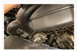
**19.** Once the MAF plate is installed, install the MAF that was removed from steps 2 & 3, use the provided hardware.
