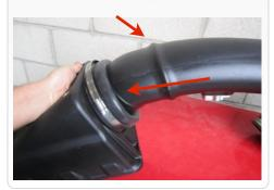
23. Once the tube is pushed flush against the stop hump of the tube the hose clamp (D) on the cuff can be tightened down. The cuff will allow some movement of the tube to accommodate engine vibration.
