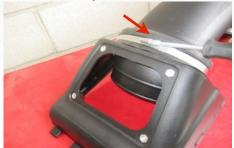
24. Install the S&B air filter (I) on to the end of the tube. Position the hose clamp (J) so that it can be accessed through the lid opening. Tighten the hose clamp.
