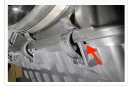
**29.** Slide the coupler (K) over the throttle body and tighten the hose clamp (L).
