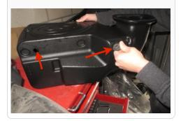
**17.** Remove the factory MAF from the factory lid using a T-30 torx.
