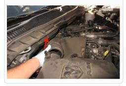
8. Remove the lid by first removing the latches on the side of the factory air box.
