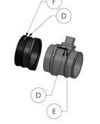
**25.** Once aligned tighten down the down clamp.
