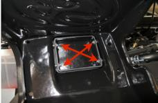
12. Move the coolant reservoir out of the way. Install the Air Box (A) using the two supplied M6x30mm screws (C) and 6mm Washers (B) for the two holes closest to the fender. Use the OE screws for the other two holes. Tighten all four.
