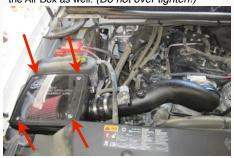
25. Re-install the engine cover. Inspect your installation, make sure the kit is properly positioned and all fasteners are secure. Reconnect the battery.
