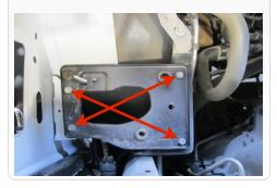
11. For those concerned about minimal engine heat; insert the four Clip Nuts (S) over the holes on the bottom opening of the Air Box (A), insert the Box Plug (T) into the end of the Air Box (A). Attach using the supplied 1/4-20 Hex Screws (U) and Flat Washers (B) from the inside of the Air box using 5/16" socket or ratcheting wrench. For those seeking additional air flow, set the Air Box End Cap aside and save all the supplied hardware. (See page 3 for more info)
