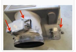
14. If equipped with Pressure Sensor, Drill a 3/8" hole using the drill point located in the Filter Adapter Tube (Y). Be careful only to drill through one surface (NOT all the way through the backside). Thoroughly clean the inside of the tube of all debris. Then install the pressure sensor using the 1/4-20 Socket Screw (N) and a 3/16" allen wrench.
