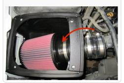
17. Install MAF sensor into the Intake Tube (AA) using the supplied 8-32x1/2" Screws (P). Do not over tighten.
