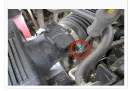
8. Using a flat blade screwdriver, remove the intake tube from the push pin located on the coolant tube. Then remove the intake from the vehicle.
