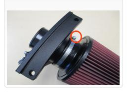
**16.** Install Filter/ Adapter assembly into the Air box.
