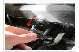
4. Disconnect the other end of the crank case vent line from the vehicle by sliding the locking tab over and pull away from the valve cover port.
