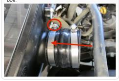
20. Secure the Silicone Step Coupler (AC) to the throttle body using a #64 Hose Clamp (F). Place the #72 Hose Clamp (G) around the top of the Silicone coupler.
