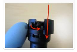
Disconnect the MAF sensor wiring harness from the MAF sensor. Note: If equipped, disconnect the Pressure Sensor wiring harness (located on the air cleaner lid) at this time as well
