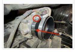
25. Insert the Intake tube assembly into the Silicone Coupler, then slide the Hump Adapter over the Adapter Tube. Tighten all hose clamps when you are satisfied with the positioning
