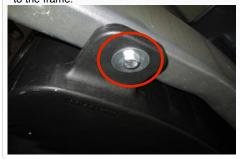
15. Insert the Air Inlet tube (S) onto the Air Box (M) and secure using the supplied 1/4"-20x3/4" screws (V), 1/4" Lock washers (U) and 1/4" Flat washers (W).
