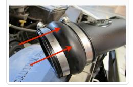
24. Secure the Silicone Step Coupler (B) to the throttle body using a #56 Hose Clamp (A). Place the #60 Hose Clamp (C) around the top of the Silicone coupler.
