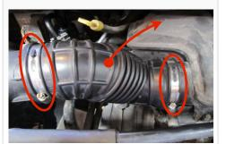
3. Loosen the two screws on the resonator assembly using a 10mm socket.
