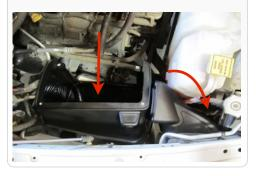
13. Using the OE bolt, secure the Air box (M) to the frame. Leave loose for now.
