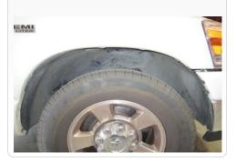
8. From inside the engine compartment, carefully pull the wiring harness connector out from the wheel liner. Then remove the wheel liner from the truck.
