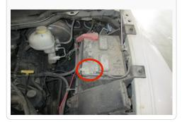
Loosen the hose clamp connecting the tube to the air box and the clamp attaching the tube to the resonator body. Then remove intake tube from the truck.
