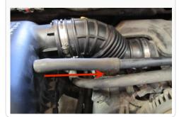
6. Remove air box by carefully pulling the air box straight up out of the four pins of the air box tray. Then remove the two bolts mounting the tray to the frame using 13mm
