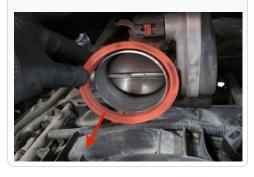
2004-08 Models: Remove the breather hose from the lid of the air box only. 2003 Models: Remove the breather hose from the oil fill reservoir.
