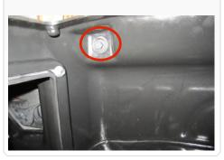
14. From inside the wheel well, attach the air box to frame using the supplied M8 x 40mm Hex bolt (K) and Fender Washer (L). Then secure both bolts mounting the air box to the frame.
