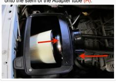
19. 2003 Models Only: Install the S&B Breather Hose (Z) onto the oil fill reservoir using the #8 Hose clamp (Y) and push the other end onto the stem of the Adapter tube
