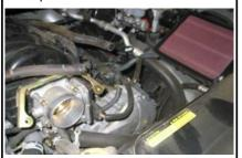
10. Remove the OE air filter from the vehicle.
