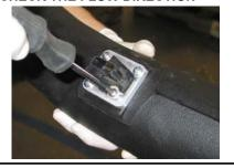
**17.** Install the intake tube and loosely secure the hose clamps.
