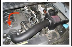
**23.** Check your installation and make sure the kit is properly positioned and all fasteners are secure. Apply the C.A.R.B. sticker in plain site under the hood. Your installation is now complete.
