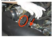
**20.** Reconnect the MAF sensor electrical connection.
