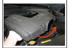
Disconnect the electrical connection for the MAF sensor.
