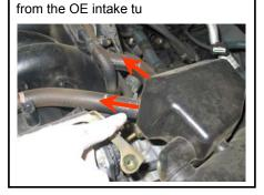
9. Remove the OE intake tube and the top of the air box.
