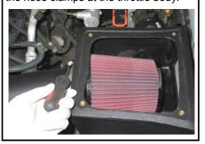
**19.** Connect both CCV lines to the intake tube.
