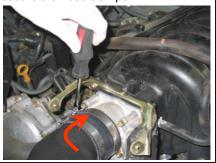
**18.** Install the S&B air filter into the air box and secure the hose clamp, secure the hose clamps at the throttle body.
