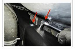
11. Attach the Mounting Bracket (F) onto the bumper mounting stud. When you are satisfied with the position, tighten the OE nut using a 18mm socket and all bracket hardware using 7/16" ratchet and socket.
