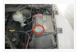
2. If you already have the S&B intake installed with the Air Inlet Plug; remove the two screws by reaching up under the truck behind the wheel liner using a 7/16" wrench to
