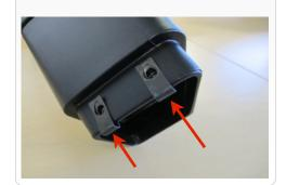
4. Secure the Mounting Bracket (F) to the Scoop (A) using the supplied 1/4-20x1.0" Screws (B), 1/4" Split Lock Washers (E) and 1/4" Flat Washers (C) on the front side and 1/4" Flat Washers (C) with 1/4-20 Lock Nuts (G) on the inside. Leave them hand tight for now.
