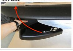
8. Slide the Scoop Assembly up into the bottom of the air box inlet channel.
