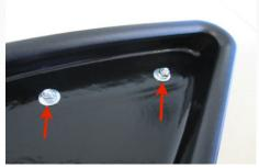
5. From under the truck; remove the bumper mounting nut using a 18mm socket.
