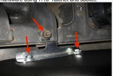
12. Check to make sure the Scoop assembly does not interfere with the wheel or wheel well liner. Turn the wheel in both directions while trying to simulate full suspension travel.
