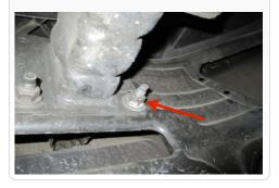
$9. \ \ \, \text{Attach the scoop channel to the air}$ inlet tube using two 1/4-20x1.0" Hex Screws (D) and 1/4" Flat Washers (F). Tighten both using a 7/16" wrench.
