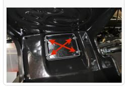
5. Loosen the four bolts mounting the air box to the truck.
