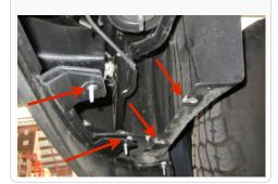
8. Slide the Scoop Assembly up into the bottom of the air box from under the vehicle. Then position the base of the scoop on top of the bumper trim tabs and wheel liner lip.
