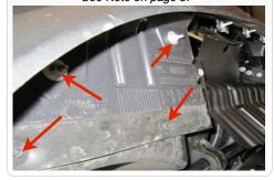
7. Remove the two clip nuts from the wheel liner and the two bolts and clip nuts from the bumper trim.
