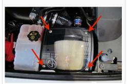
15. Reconnect the negative battery terminal. Inspect the installation, be sure the kit is properly positioned and all fasteners are secure.
