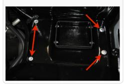
6. From under the truck; remove the two screws mounting and the two nuts mounting the plastic shield. Save this piece so it can be reinstalled during heavy rain and snow. See Note on page 3.
