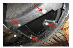
12. Tighten down the four screws in the bottom of the air box.
