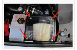
3. Loosen both hose clamps on the hump adapter and the slide the hump adapter over the adapter tube. Loosen clamp and slide intake tube out of the turbo adapter. Then remove the Adapter tube and Air Filter from the air box
