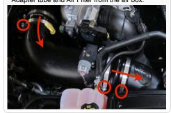
4. If installed, remove the air box plug from the air box. If not, install the three clip nuts that were supplied with the intake kit onto the bottom opening lip of the air box.
