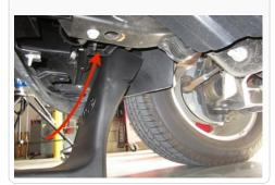
$9. \ \ \, \text{From inside the air box grab the top of the}$ Scoop assembly and align with the four holes in the air box. Note: It may be necessary to move some wiring harnesses out of the way to gain
